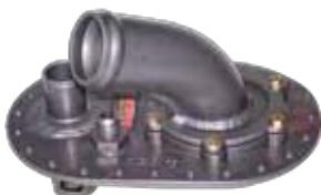
NASCAR® Billet Fill Plate SFI 32.2 approved with high flow fill valve, ultra lightweight, anodized Part No. NASCOT-5P2
