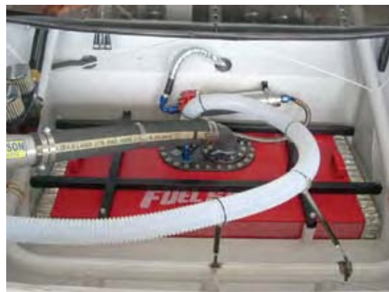
NASCAR® Billet Fill Plate SFI 32.2 approved with high flow fill valve, ultra lightweight, anodized Part No. NASCOT-5P2
